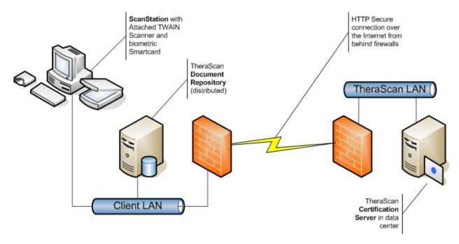
**ScanStation:** This is the PC or thin client that will run the web-based application used to scan, load and sign the source-document copies. Therapeias recommends TWAIN scanners from Canon and Fujitsu.
